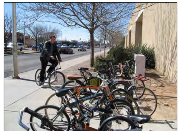
Bicycle rack designs should include racks that provide two two points of contact with the bicycle so that it can be locked from both the front wheel/frame and the rear wheel.
